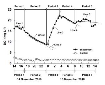
**Figure 3:** A typical example of the diurnal DO fluctuations monitored every thirty minutes between 14:00 on 14 November and 15:00 on 15 November 2018. They were divided into five different periods (Period 1 to Period 5), and a regression line was interpolated to the data plots in each of the five periods.
